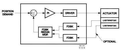
**Typical Integrating Actuator Block Diagram**
