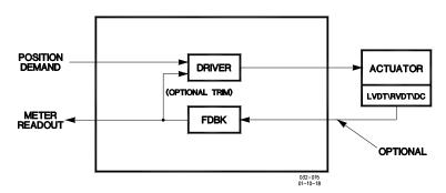
**Typical Proportional Actuator Block Diagram**
